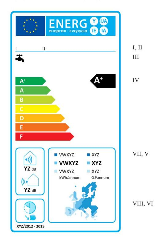
1.2.3. Heat pump water heaters in water heating energy efficiency classes A<sup>+</sup> to F
