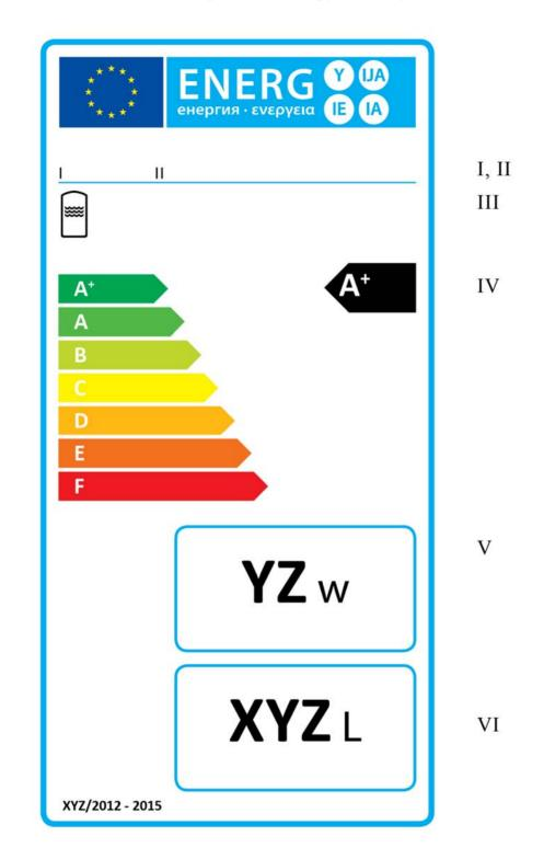
2.2. Label 2 for hot water storage tanks in energy efficiency classes  $A^+$  to F
