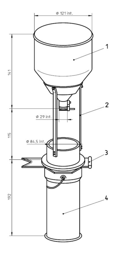
**Key** 1 Filling hopper 2 Funnel supports 3 Cut-off blade 4 Measuring container, capacity 1 litre
