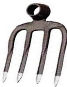
Figure 6 — Fork hoe with four tines
