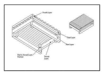
0.75- by 0.75-inch (19- by 19-mm) kindling fuel into the inside of each corner using 18 gage by 1.25 inch (32 mm) brads.
