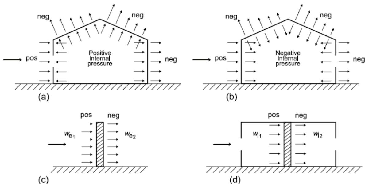
Figure 5 - Pressure on surfaces
