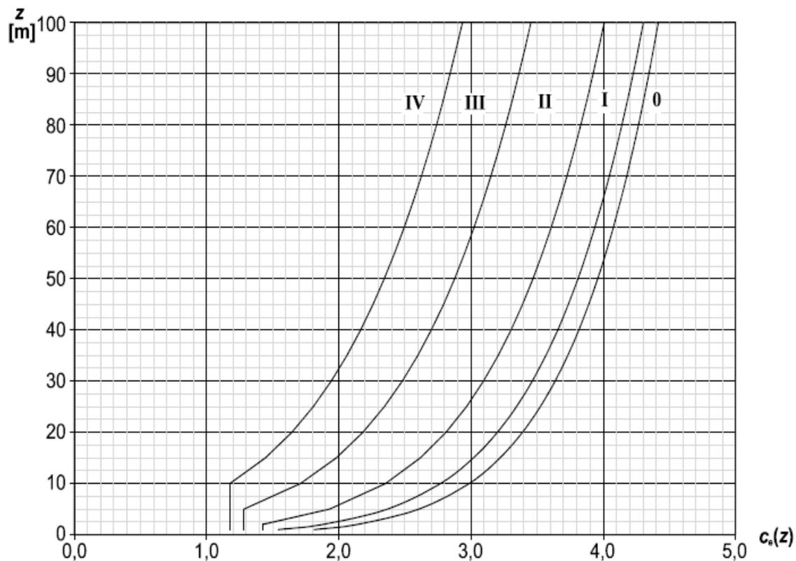
**Figure 3 — Illustration of the exposure factor  $c_e(z)$  for  $C_o = 1.0$ ,  $K_r = 1.0$**
