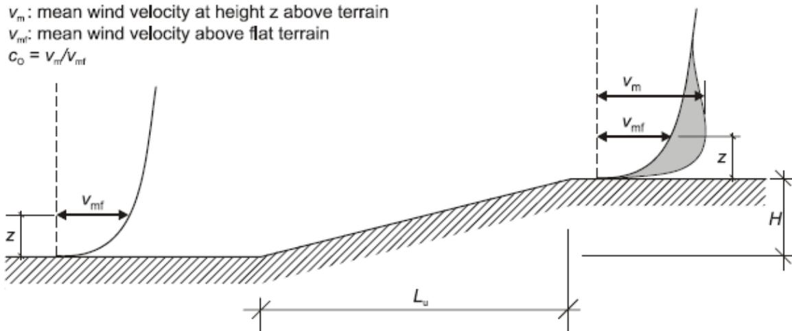
Figure 2 - Illustration of increase of wind velocities over topography
