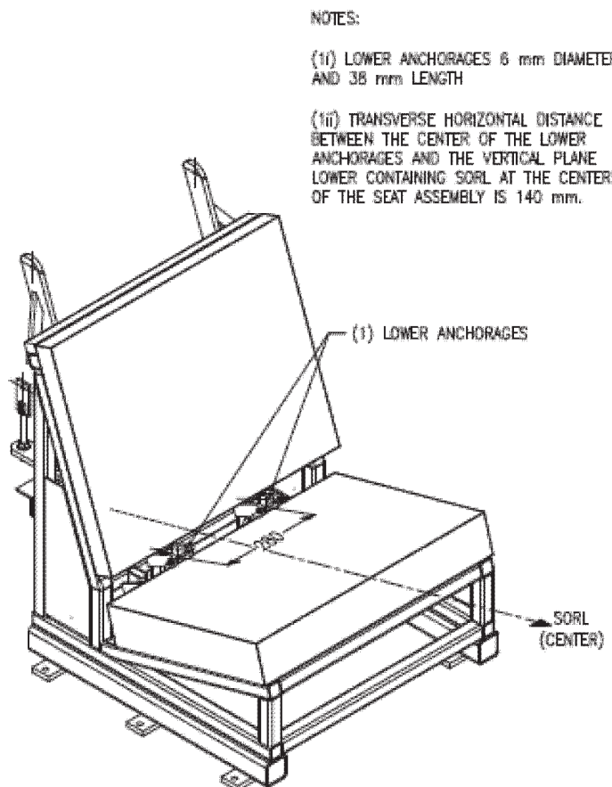
SEAT ORIENTATION REFERENCE LINE AND LOCATION OF THE LOWER ANCHORAGES OF THE CHILD RESTRAINT ANCHORAGE SYSTEM ON THE STANDARD SEAT ASSEMBLY
