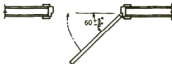
Figure 8 — Typical arrangement of slamming test
