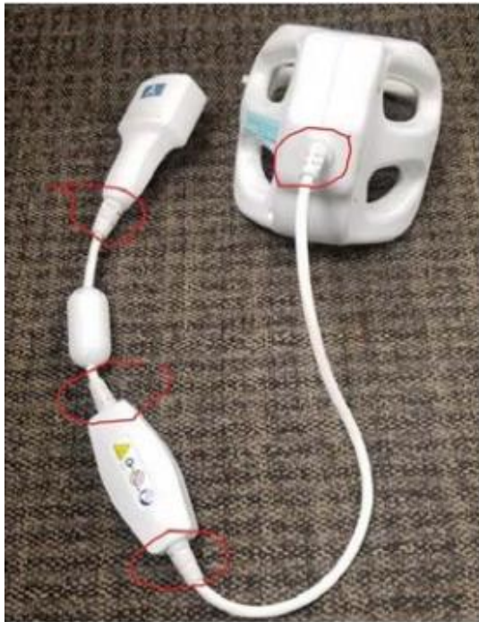
Figure 1: MRI Coil for the shoulder; the four strain relief boots are circled in red. Source: GE Healthcare Application.
