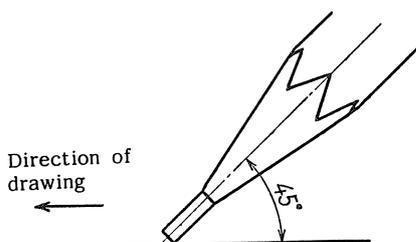
**Figure 3 — Pencil hardness testing method**
