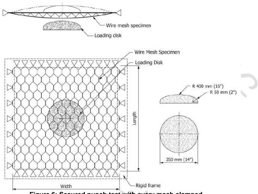
Figure 6: Secured punch test with every mesh clamped
